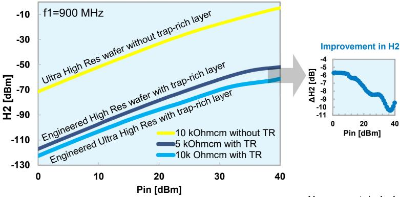
Using 10 kOhmcm crystal with TR layer as opposed to 5 kOhmcm, even 10 dB further improvement in linearity can be achieved especially at high powers.
