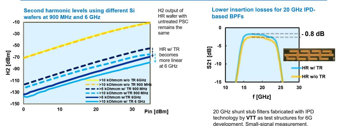
Measurements by Incize. 2 mm length 50  $\Omega$  CPW test structures.
