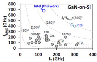
Fig.16 benchmarks the  $f_T/f_{MAX}$  of this work with data points reported [13] for GaN-on-Si transistors, showing record  $f_{MAX}$ =680GHz with  $f_T$ =130GHz, shown in Fig.12. Intel data points are the only ones from 300mm GaN-on-Si(111) process.
