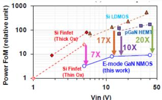
Fig.11 benchmarks the power FoM of the e-mode GaN NMOS of this work, showing ~20X better performance than pGaN HEMT and ~30X better than Si LDMOS at 40V; 10-17X better than Si LDMOS and pGaN HEMT at 12-15V, and 7X better than Si Finfet at 5V.
