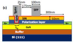
E-mode high-K GaN Transistor (Source Field-Plate)
