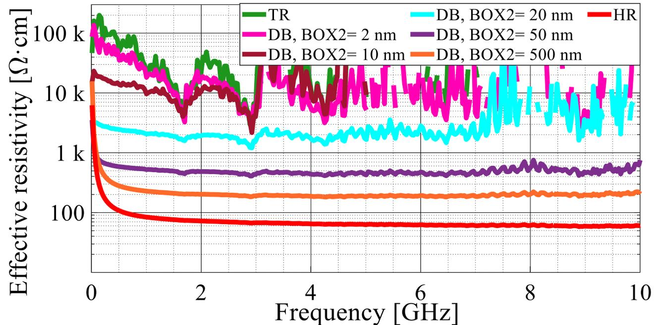
Measured effective resistivity as a function of the frequency for the TR, HR and DB substrates with different BOX2 thicknesses.
