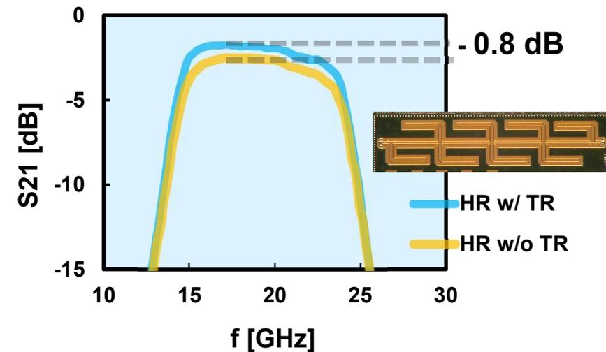
20 GHz shunt stub filters fabricated with IPD technology by VTT as test structures for 6G development. Small-signal measurement.
